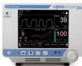
Figure 1. Capnograph: monitoring \text{ETCO}_2 (39 mmHg, graph with exhalation plateau; pulse oximetry with RR 8, \text{SpO}_2 100%)
